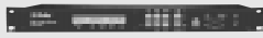
DP503 encoder provides MPEG Layer II coding as well as both Dolby AC-2 and Dolby AC-3.
