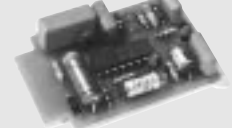
Signetics' B-type IC made it easier to incorporate Dolby NR in consumer products.
