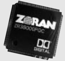
Zoran introduces first single-chip processor capable of Dolby AC-3 digital audio coding and decoding. First used in second-generation DA20 Dolby Digital film sound adapter.
