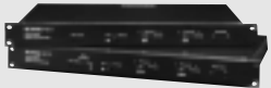
DP500 Series codecs were the first to utilize the Dolby AC-2 algorithm.
